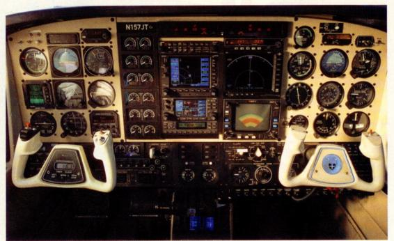
Wide-chord. four-blade Hartzell propellers (above) provide tremendous thrust and low vibration while maintaining adequate ground clearance. A new Moritz electronic engine instrument cluster (left), a custom annunciator panel, and a Shadin **ETM trend** monitor/air data computer are a major part of the **Royal Turbine** treatment.
